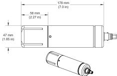
Dimensions for the stainless steel RDOX sensor:
